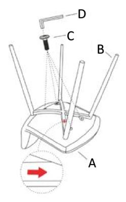
Attach Seat Legs (B) to Seat (A) with Bolt (C) using Allen Key (D)
